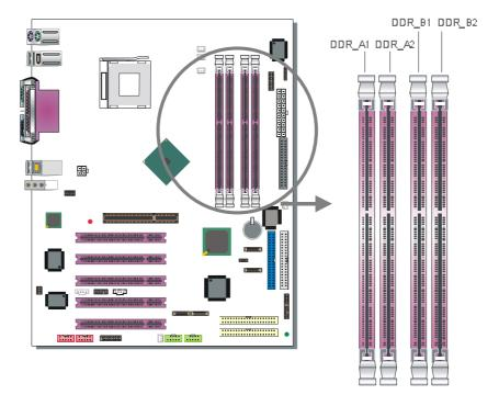
This motherboard supports two Dual Channels to your memory. Note that you can use normal DDR memory for Dual Channel to work. Also note that for Dual Channel to work 2 or 4 modules of equal size and specifications have to be installed.
